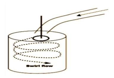
Fig.1: swirling motion in an engine cylinder
