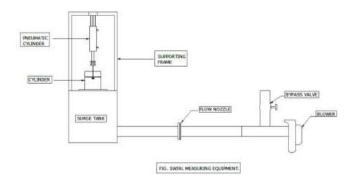
Fig.2: Block diagram of swirl measuring equipment experimental set up
