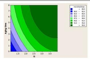
Fig.3 Effect of TI and Aging Time on Micro Hardness
