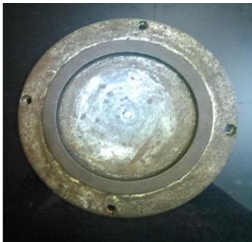
Fig.2 Show the wear samples of CADI 8mm diameter and counter face wear base plate
