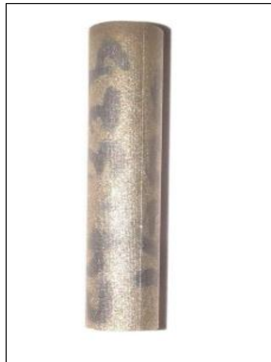
Fig.2 Show the wear samples of CADI 8mm diameter and counter face wear base plate
