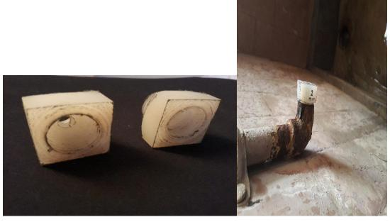
Here, we have used 5 tests nozzles with inner diameter (d2) as 2mm, 4mm, 6mm, 8mm, 10mm.
