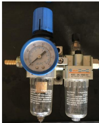
Figure 5. FRL Unit (Filter RegulatorLubricator)
