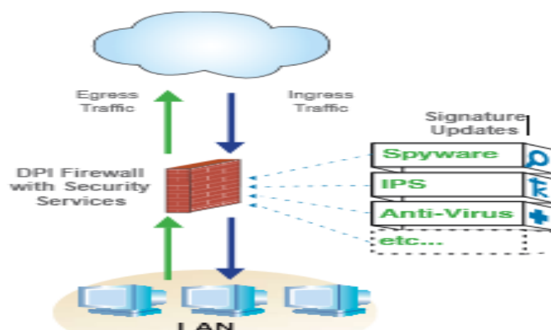
Fig. 2 The security appliance is now a dynamic system that requires regular signature updates
