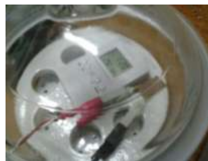
Fig 2Sensor holding connection with LCR and Humidity meter
