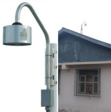
Figure 1 Electric Field Mill as installed in the University of Kashmir.
