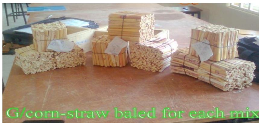
Figure 2.2: Straw Bale Samples.
