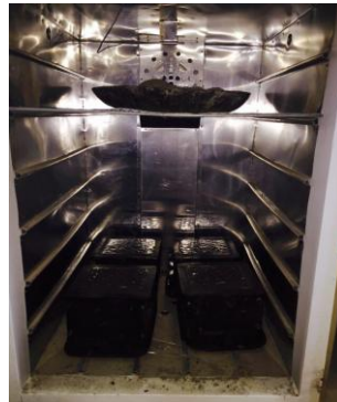
Figure.2 Curing of Geopolymer Concrete Specimen
