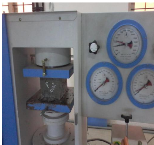
Figure.5 Compression Testing of Geopolymer Concrete Cube
